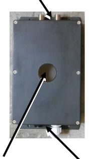
1.5" dia. clear acrylic window for built-in, rugged, concealed 5 mega-pixel Forward *Pivot™* micro PTZ color camera
