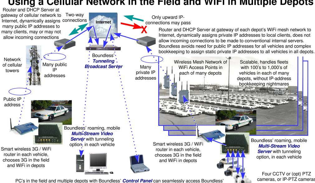
Multi-Stream Video Servers that use 3G cellular in the field and WiFi in depots, via Boundless' Tunneling Broadcast Server, regardless of location, networks' routability, IP addresses and changes in IP addresses
